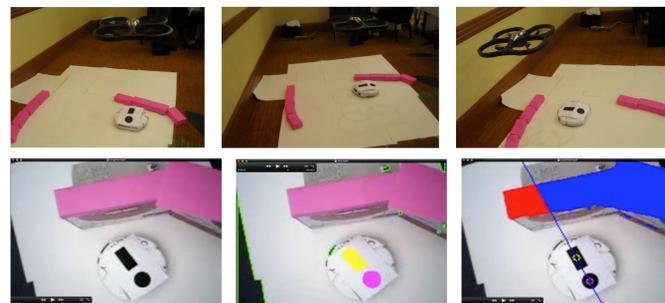
**Mutual support:** (top) An iRobot Create leads an ARDrone up to an obstacle; the drone's overhead view then provides the correct direction to navigate (bottom) the factorial-finding sensing routines via image segmentation
