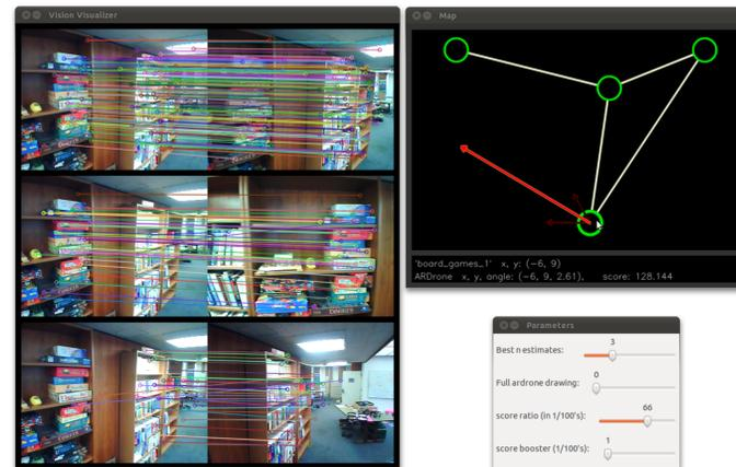
The team's user interface showing the top three map matches for the current live frame (left), the location graph and pose estimates (top right), and (bottom right) a control panel with the system's localization parameters.
