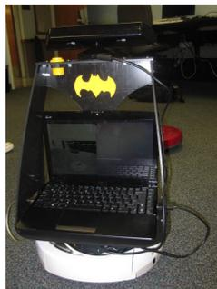
This project explored the capabilities of the inexpensive (\$300) Parrot ARDrone, a quadrotor helicopter. The iRobot Create was the foundation for our ground robots. The ARDrone is quite sensitive to its surroundings, and it requires careful scaffolding to move deliberately and autonomously. The Create offers an extensible base for a Kinect, laptop, and shelf, a variant on M. Ferguson's design.
