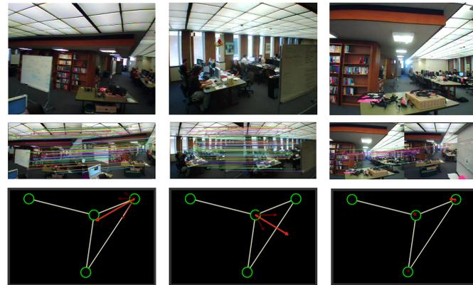
**SURF-based localization:** (top) trial input images in Sprague (middle) best-matching SURF features (bottom) the localization interface with the drone's pose estimates
